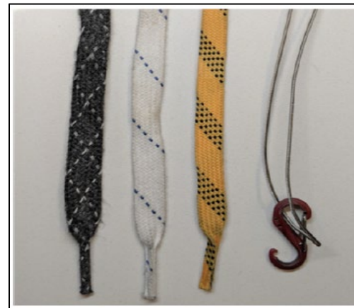
Figure 2. Three laces used for stiffness assessment. Left to right: carbon fiber blend, non-waxed, waxed, and cable.
